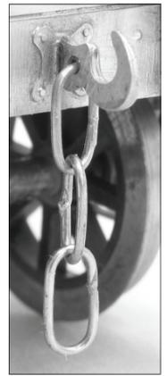
Pass the coupling hook through the slot and retain it with a length of spring wire. Polish the centre of this wire with emery cloth first so that you can solder it to the coupling hook shank once you are happy that the buffers spring freely.
