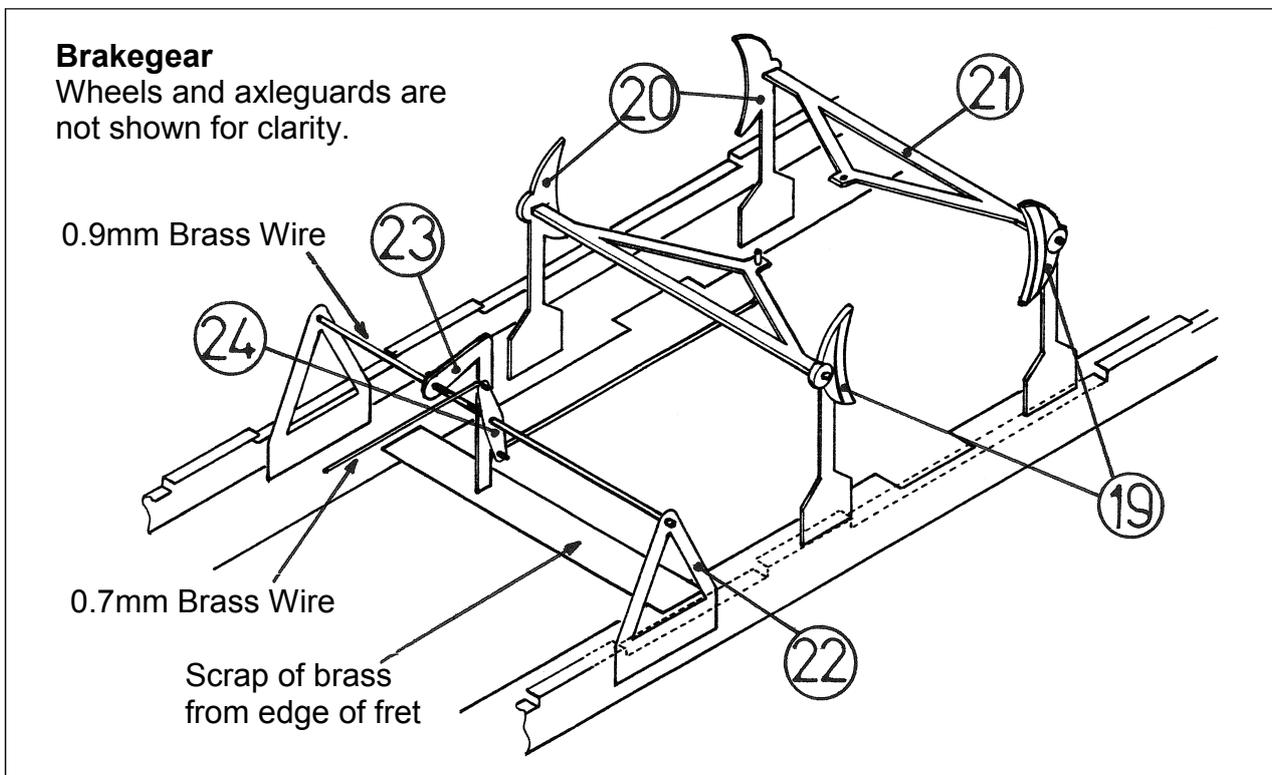
6. Solder brake blocks (parts 19) to brake hangers (parts 20) making up four L/H and four R/H. Then fit into slots to line up with the wheels. I find it useful to hold them with miniature crocodile clips.
