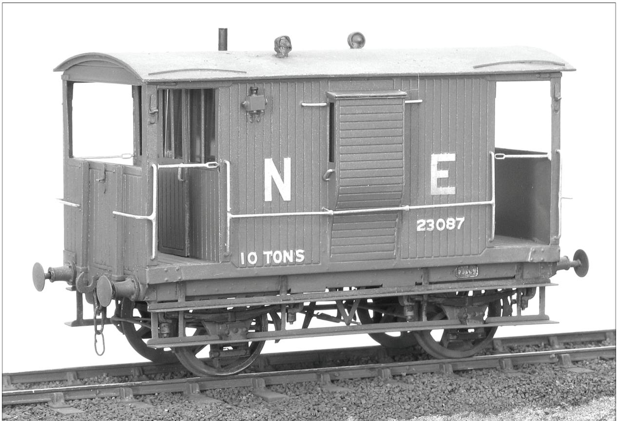
**PROTOTYPE.** This diagram was the last design of goods brake van built by the NER. Many of the constructional features found their way into the LNER standard design. After grouping the brakes could and often did work all over the LNER system. A number lasted into BR days.
