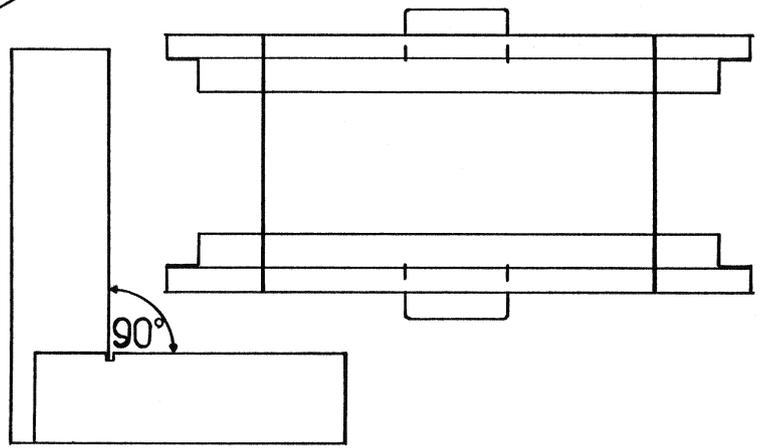
3. I now detail up the body. Fit the corner strapping (parts 12). Fit to the ends first locating the etched packing ring over the buffer hole and then bend around the sides.
