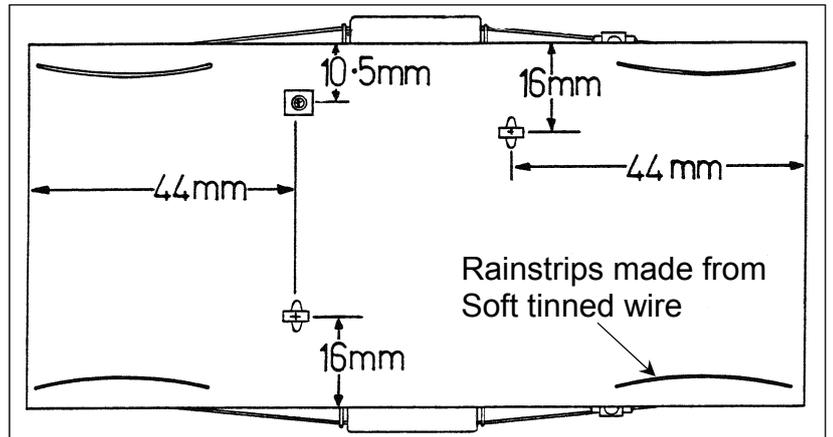
It is intended that after painting the roof is glued into place with Evostick, used as a contact adhesive (follow the instructions on the tube) but if you wish to have a removable roof, solder tabs made from waste etch to the underside of the roof so that they will clip inside the cabin body.
