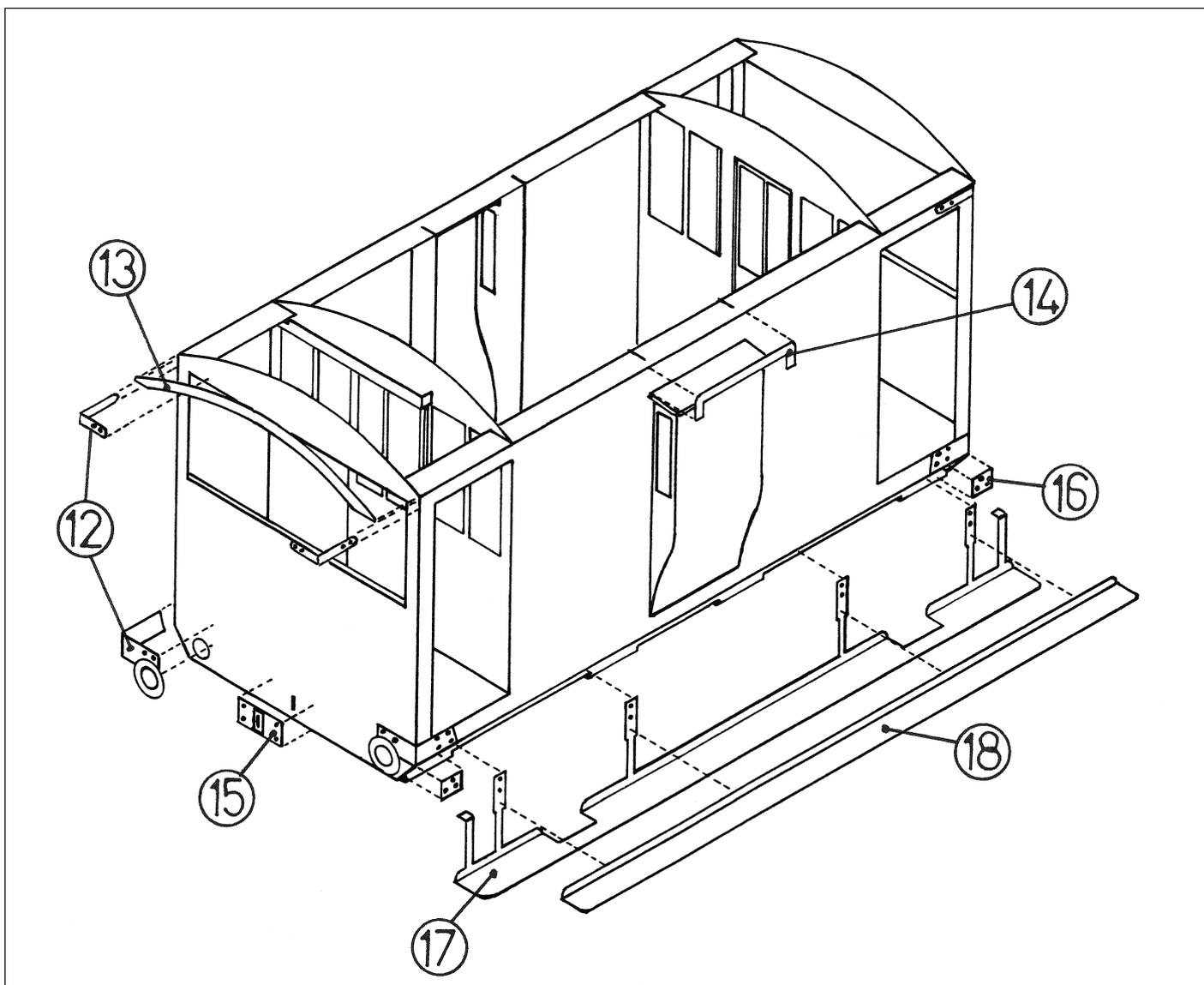
4. Fit corner reinforcing plates (parts 16) to solebars. Then fold up lower foot boards (parts 17) and fit to solebar (Note etched marks on solebars to help with positioning of footboard supports). Then fold up and fit the upper footboards (parts 18) locating onto the footboard supports with etched rebates.
