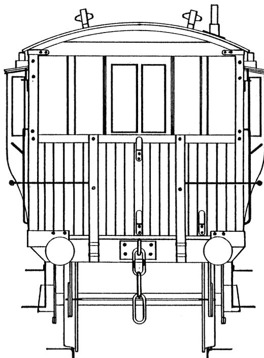
**Livery, Bodywork** - Red Oxide. Buffer beams, solebars, footboards and running gear - Black. Roof - White lead (probably better as dirty grey). Veranda floor - Dirty wood (Humbrol 110). Lettering - White.
